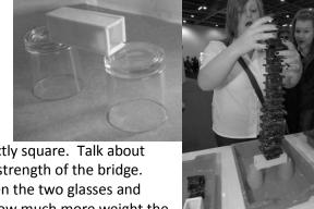
causing the beam not to be perfectly square. Talk about how these factors may affect the strength of the bridge. Then, place the box girder between the two glasses and begin to load with weights. See how much more weight the box girder can take than the plank before it breaks.
