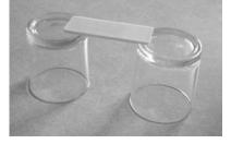
take them out of the rolls in order to add weight that is light enough for the plank to support. Take note of how much weight you loaded when the bridge breaks.
